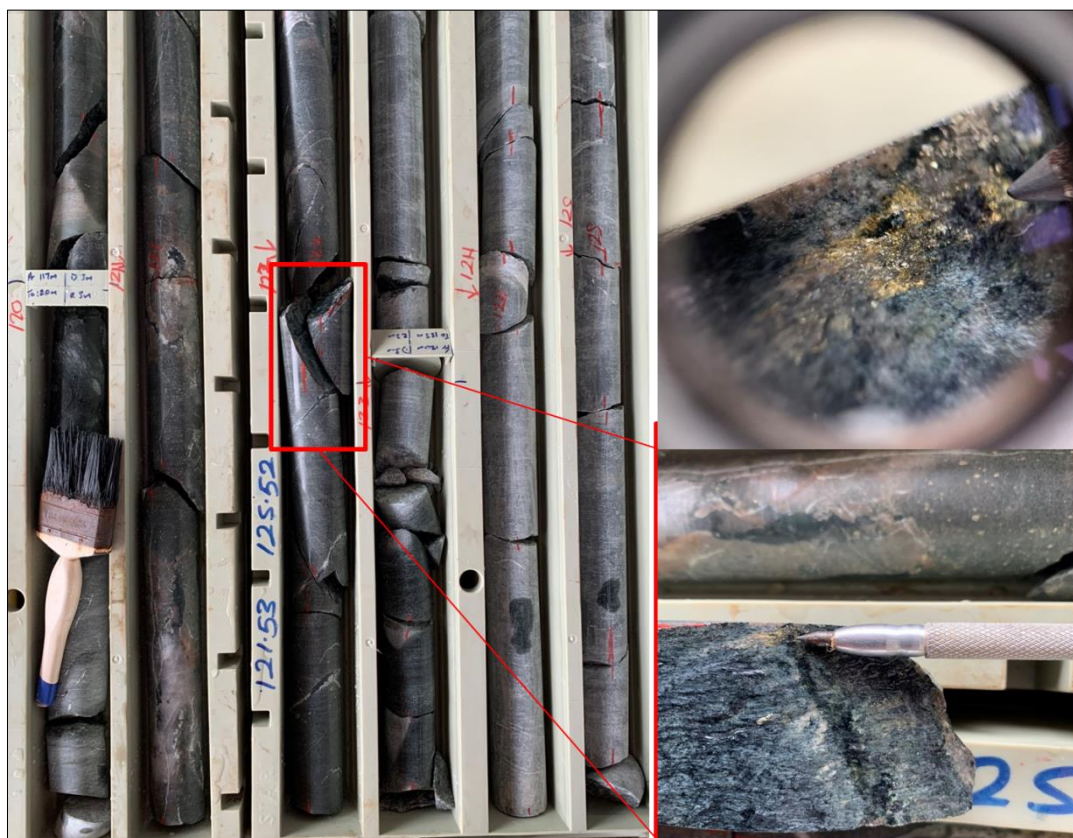
Figure 3: High-grade gold mineralisation in SDD196 from 119.5m to 125.5m with strong silica+albite alteration, euhedral coarse pyrite and visible gold at 121.95m.
