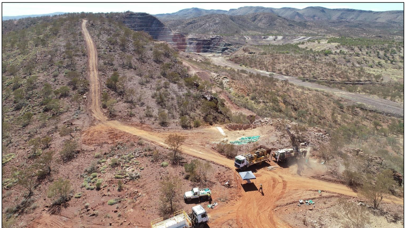
Figure 2: RC drilling at Connie's Find, approximately 400m to the west of the Waugh Pit shown in the background
