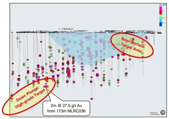
Figure 3: Long Section highlighting the 2 target areas presently being drilled at Mon Ami
