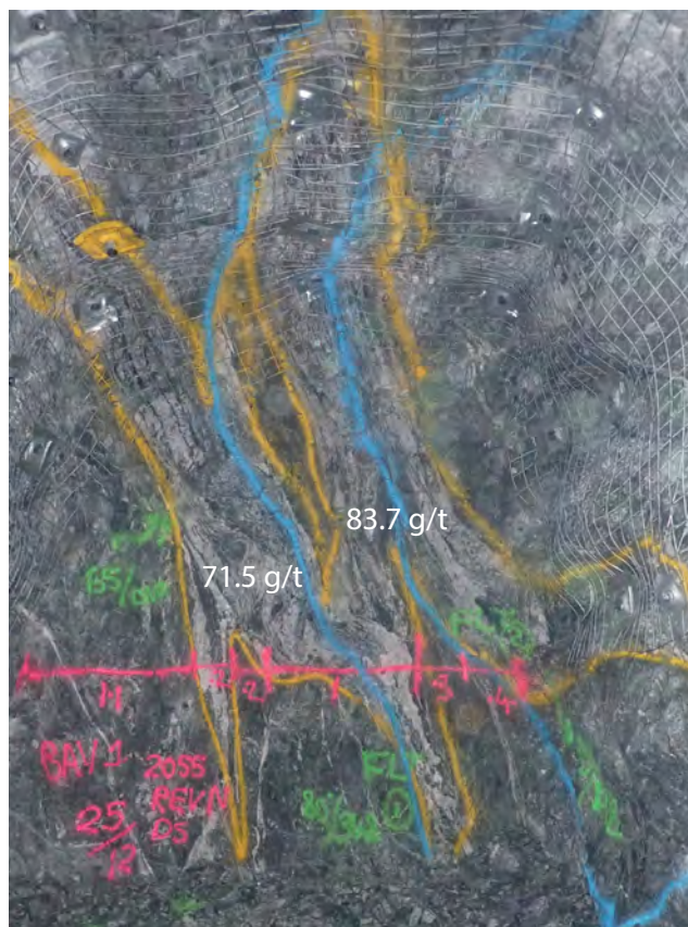
REV splay lode being developed on the 2055 level with weighted average face grades of 3.0 m @ 20.37 and 3.2 m @ 24.42 g/t
