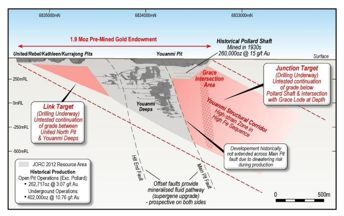
Figure 1 - The Grace-Mine shear zone intersection below the southern half of Main Pit i.e. "Junction Target".
