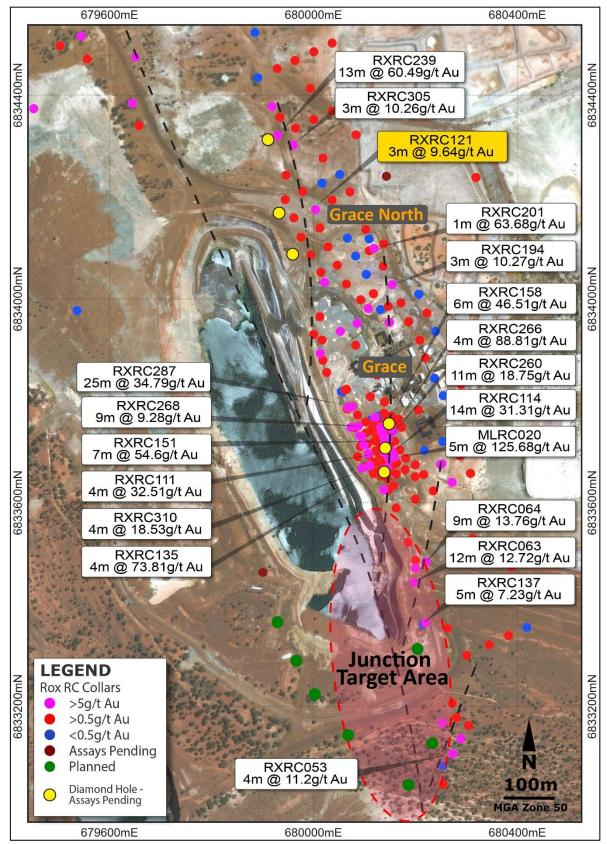
Figure 5 – RC and Diamond Drill hole collars and intercepts over Aerial Photo.
