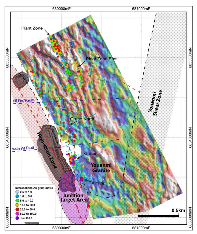
Figure 4 - First Vertical Derivative of magnetometric conductivity (MMC). SAM survey.
