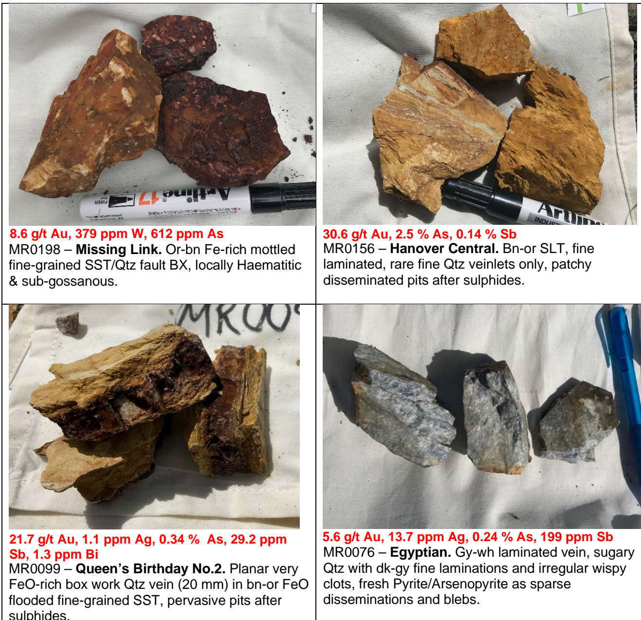
Figure 7: Selection of high grade rockchip samples from the Stage 1 dump sampling program on the Drummond and Belltopper fields. Samples include mineralised breccias, altered siltstones with minor quartz veining and a several quartz vein types. (Abbreviations: Qtz - Quartz, SST - sandstone, SLT - siltstone)
