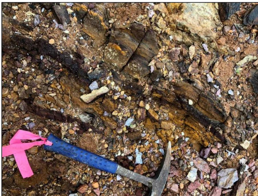
Achilles 2: photo of outcropping massive Sulphide vein at Achilles 2 gravel quarry
