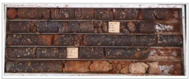
Figure 5:6 High Grade (>20% Mn) Mineralisation in Drillhole JDDH01
