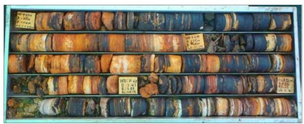
Figure 5:7 Medium Grade (>14%Mn) Mineralisation in Drillhole JDDH01 Source: Wamex a95026
