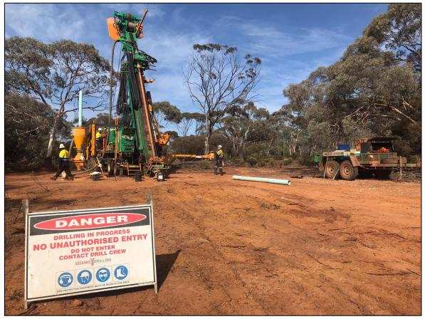
Photograph 1 - Reverse Circulation drilling at the Nepean Nickel Project
