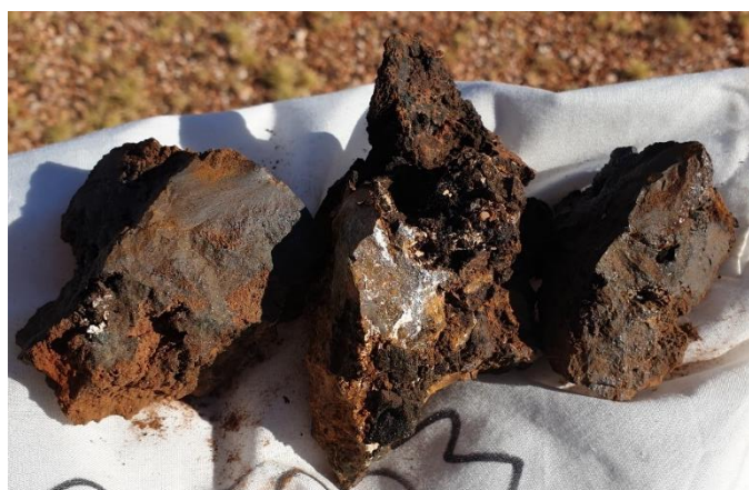
Figure 7: Photograph of gossan sample RT003 that returned 3.6 g/t Au. Note classic black boxwork textures particularly in the middle sample that look semi-massive.
