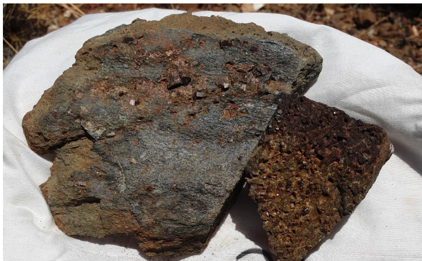
Figure 9: Photograph of chlorite-pyrite-altered sheared mafic sample RT026 that returned 1.5 g/t Au. Note abundant cubic pyrite throughout
