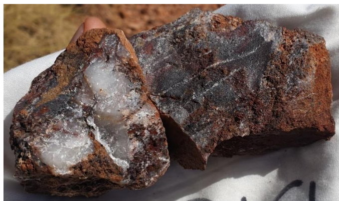
Figure 5: Photograph of chert/BIF with quartz veins and gossan from sample RT019 that returned 0.8 g/t Au.
