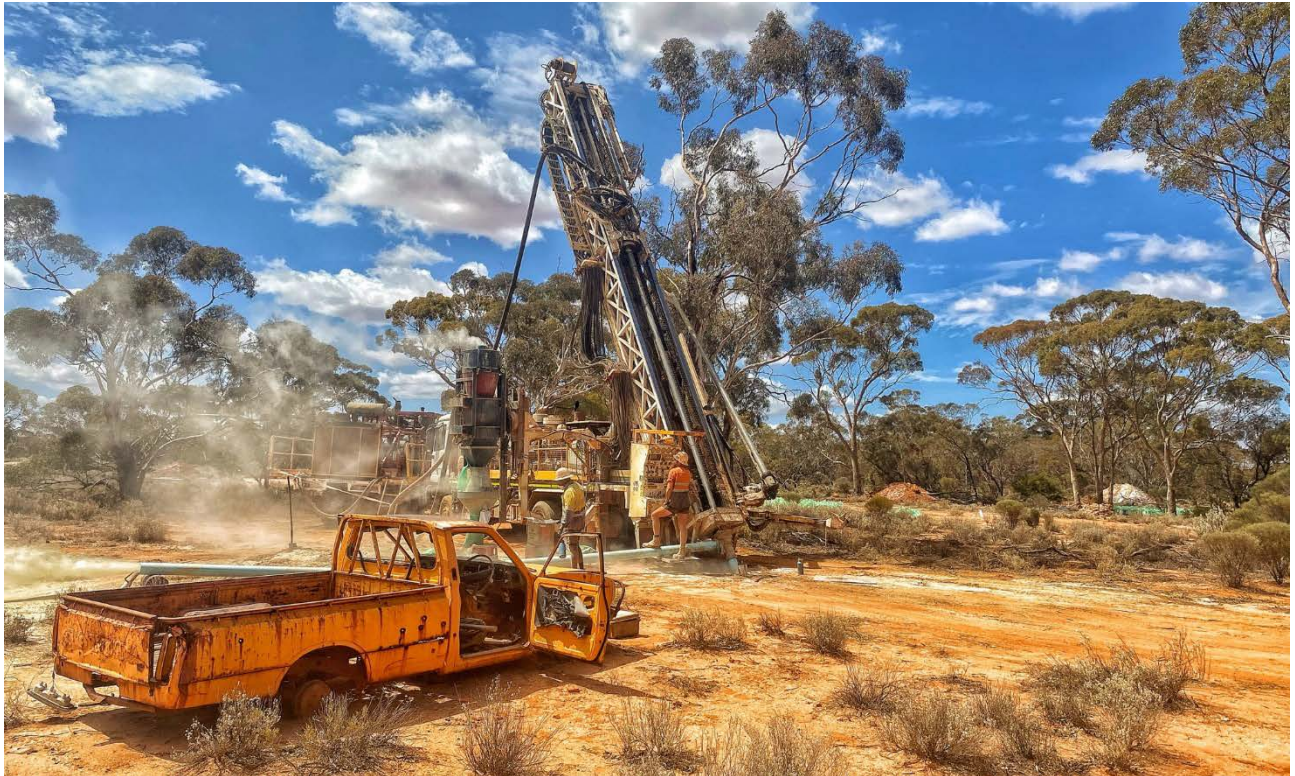
Figure 1: RC drilling at Rowe's Find during December 2020. Photo courtesy of Raglan Drilling (vehicle in foreground not currently in use)
