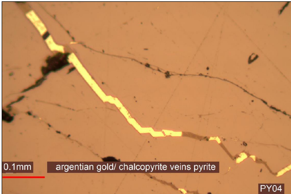
Figure 3 – Part of polished thin section showing silver-bearing (argentic) gold vein (yellow) from NE Bankan cutting through pyrite (iron sulphide) - from DD hole KKODD009, 152.0m
