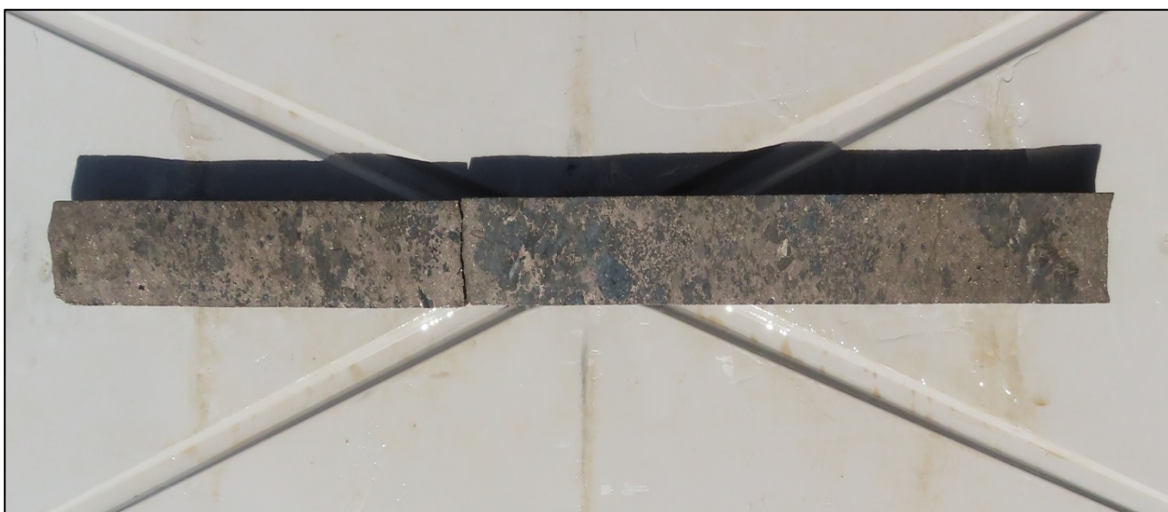
Photo 2: ANDD0011 – Semi-massive to massive Ni-Cu sulphides @ 33.1m – 33.8m
