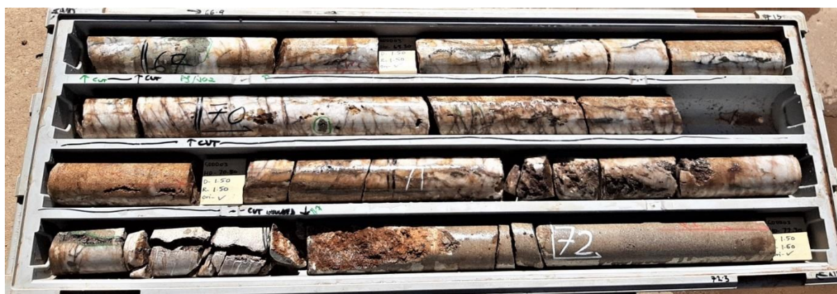
Figure 11 – Gordons Dam diamond drill core hole YRLDD007 from 68.90m – 72.30m downhole showing a fractured and brecciated quartz vein interspersed with coarse pyrite and minor chalcopyrite – assay results pending. Note the low angle to core axis contact with a granite porphyry unit at approximately 71.50m.
