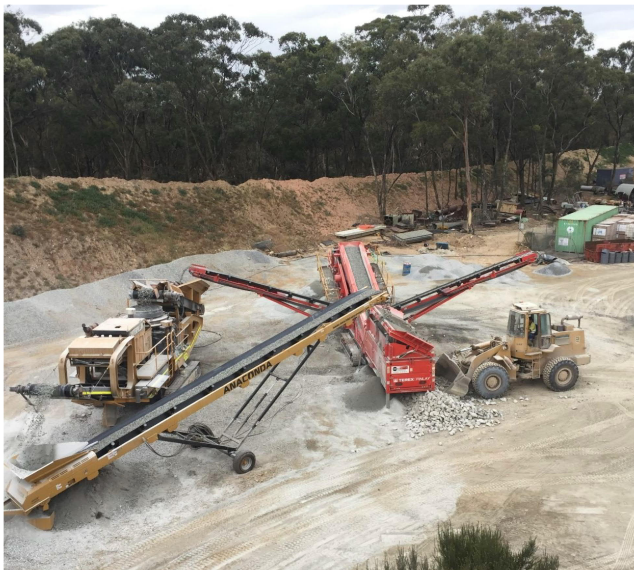
Figure 2. Secondary 'Cone' Crusher, screen and grizzly, Porcupine Flat Processing Facility.
