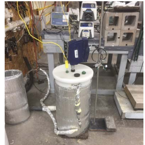
Image 2 – Hazen Laboratories Bulk Neutralisation Process
