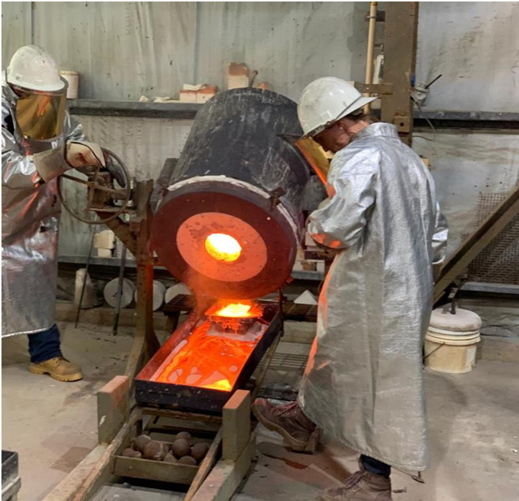
Figure 2: Pouring Gold at the Maldon Processing Plant
