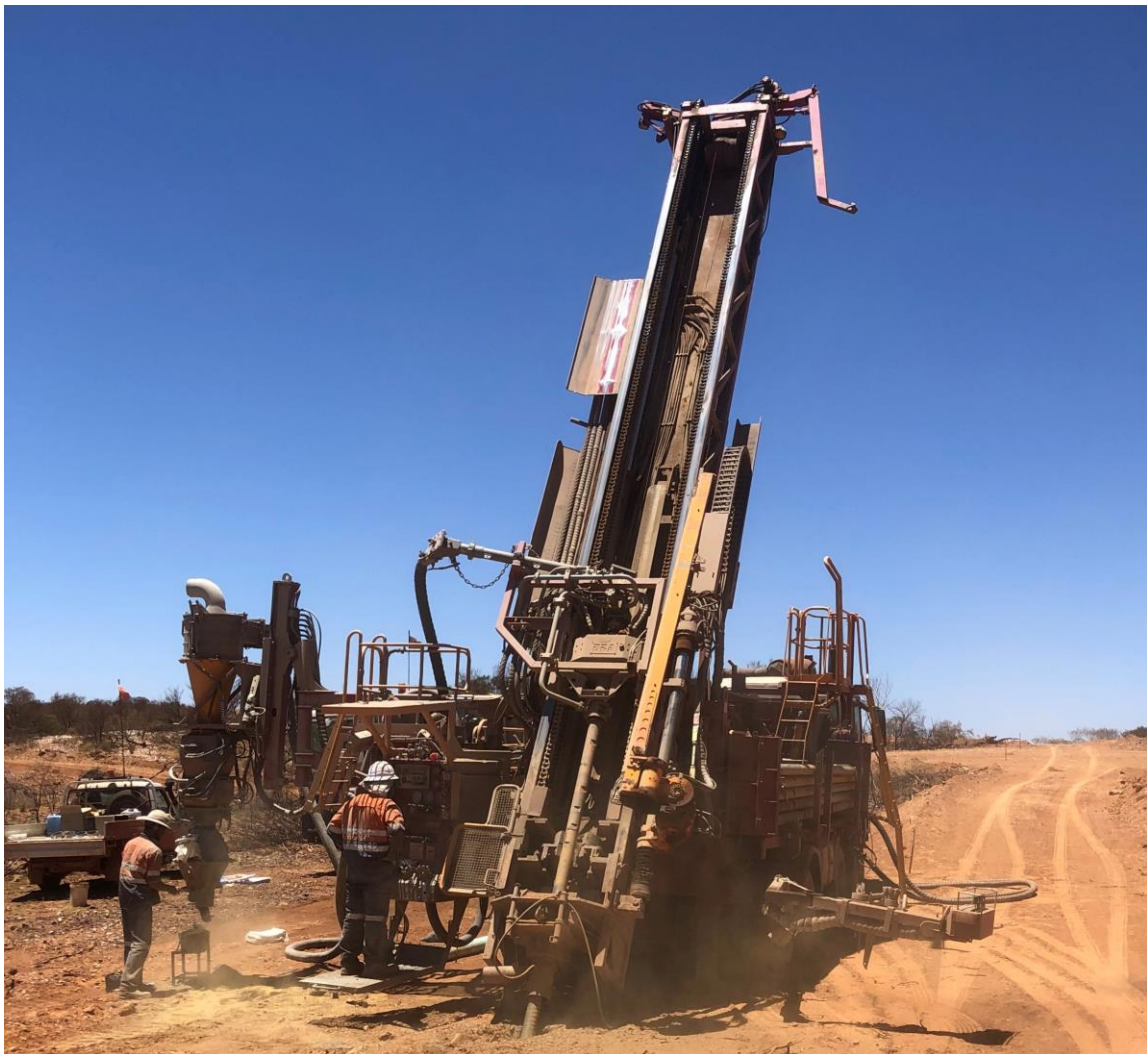
Figure 4: The RC Rig collaring at Saltwater mining area in preparation for drilling, targeting old worked areas from the 1980s.
