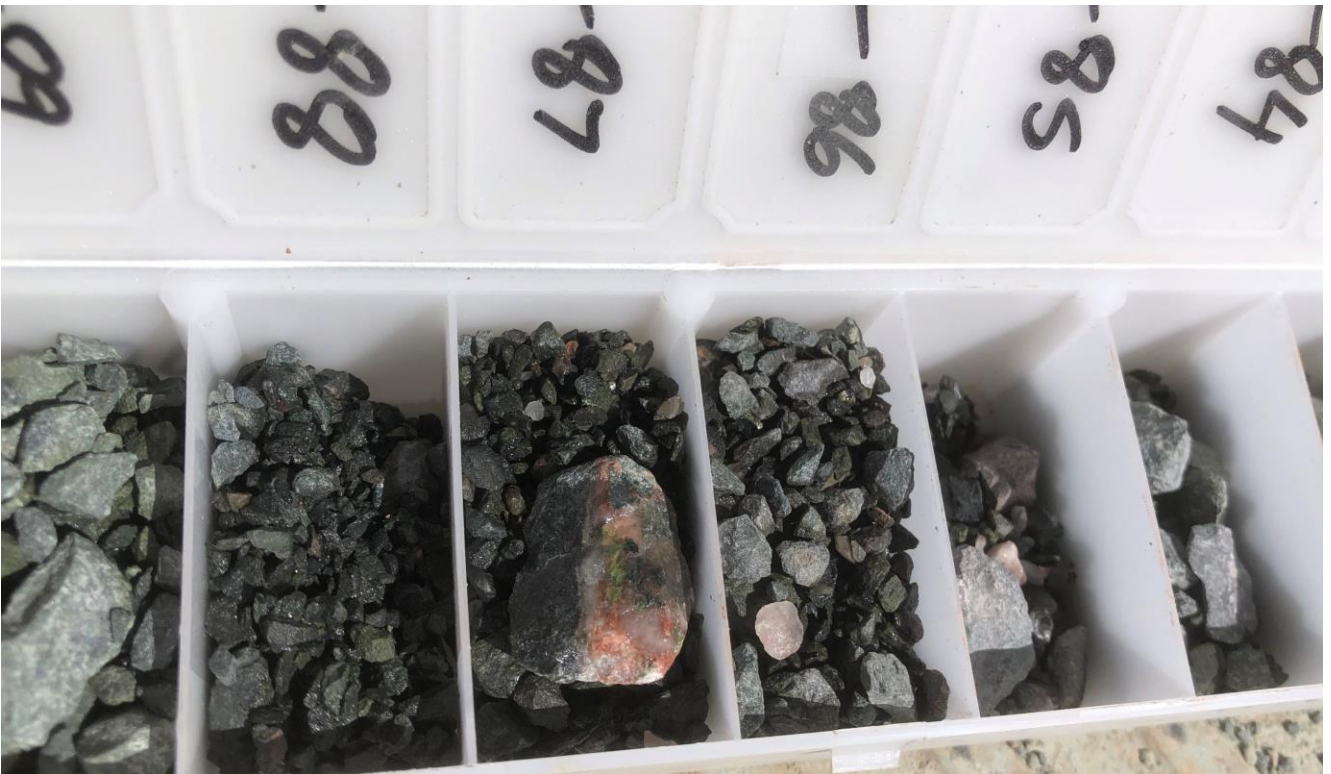
Figure 6: Samples from drill hole SWRC15 showing alteration and sulphides at 84 to 88m down hole.
