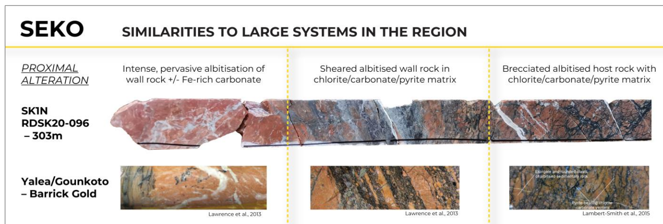
Figure 2: Comparison of alteration styles from the SK1 North (top) and Yalea/Goukoto (bottom) gold deposits 1,2
