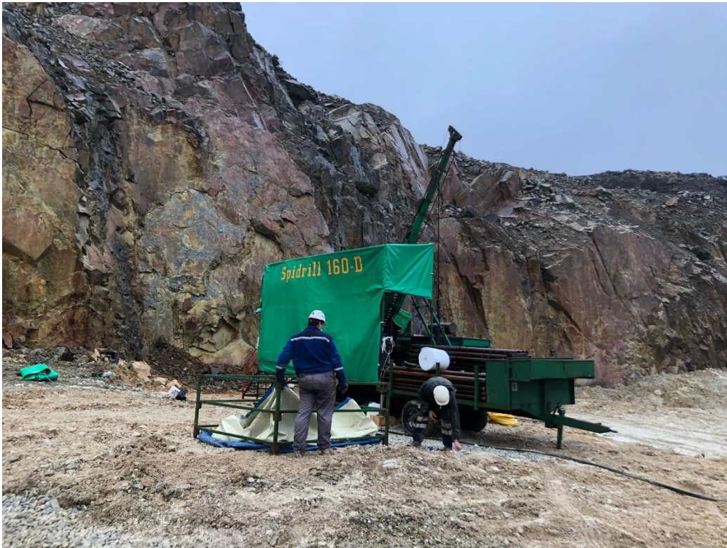
Figure 2 - Spidrill 160D diamond drill rig at MC108
