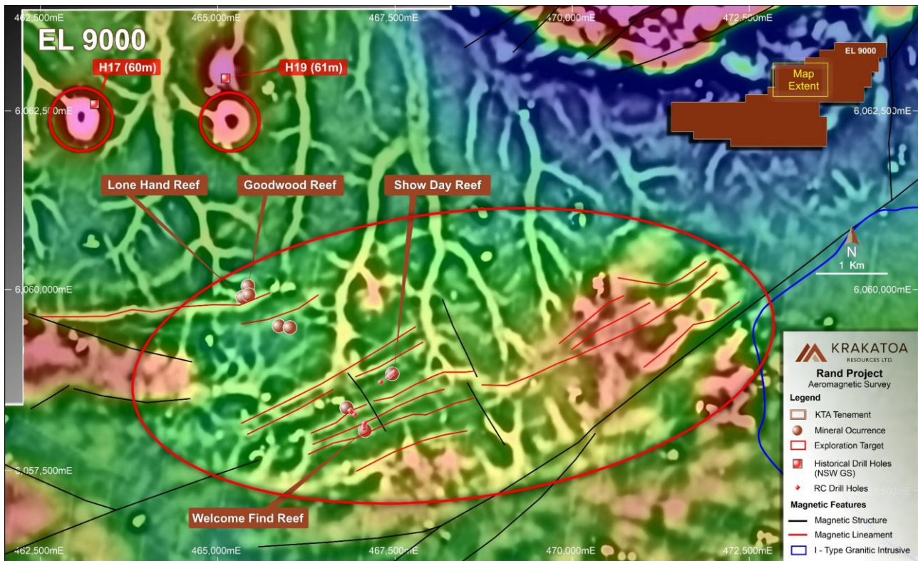
Figure 3 – Detailed section around the Bulgandry Goldfield. Note the NE-trending magnetic lineaments, not seen before, associated with the prospecting gold locations; the well-preserved palaeochannels; and, the recognition of different intrusive bodies based on the geophysical response.
