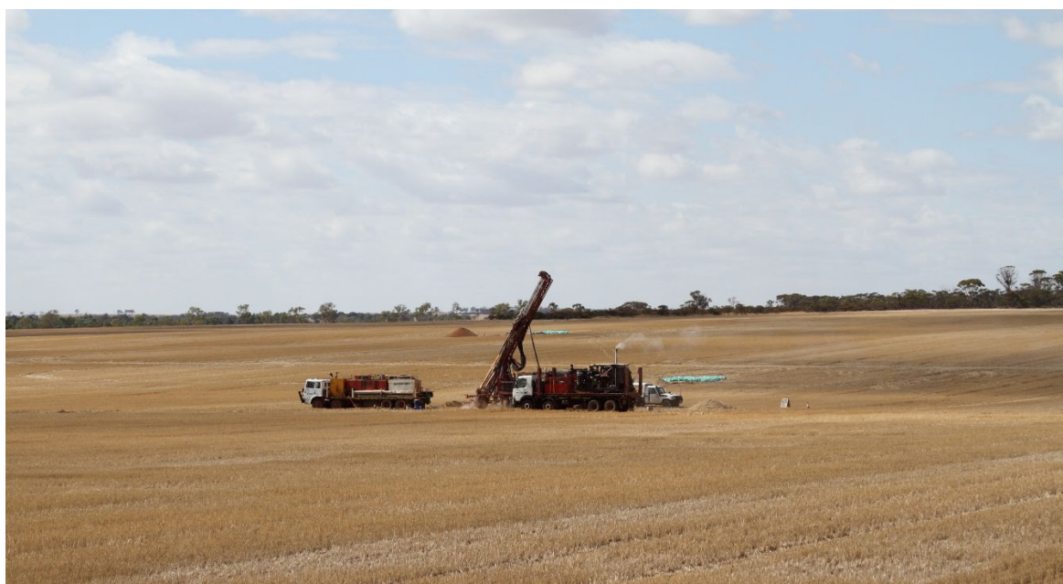
Figure 1: Bindi deposit infill RC percussion drilling in progress at hole 21CARC010 on section approximately 100m south of hole 21CARC002 (25 January 2021).
