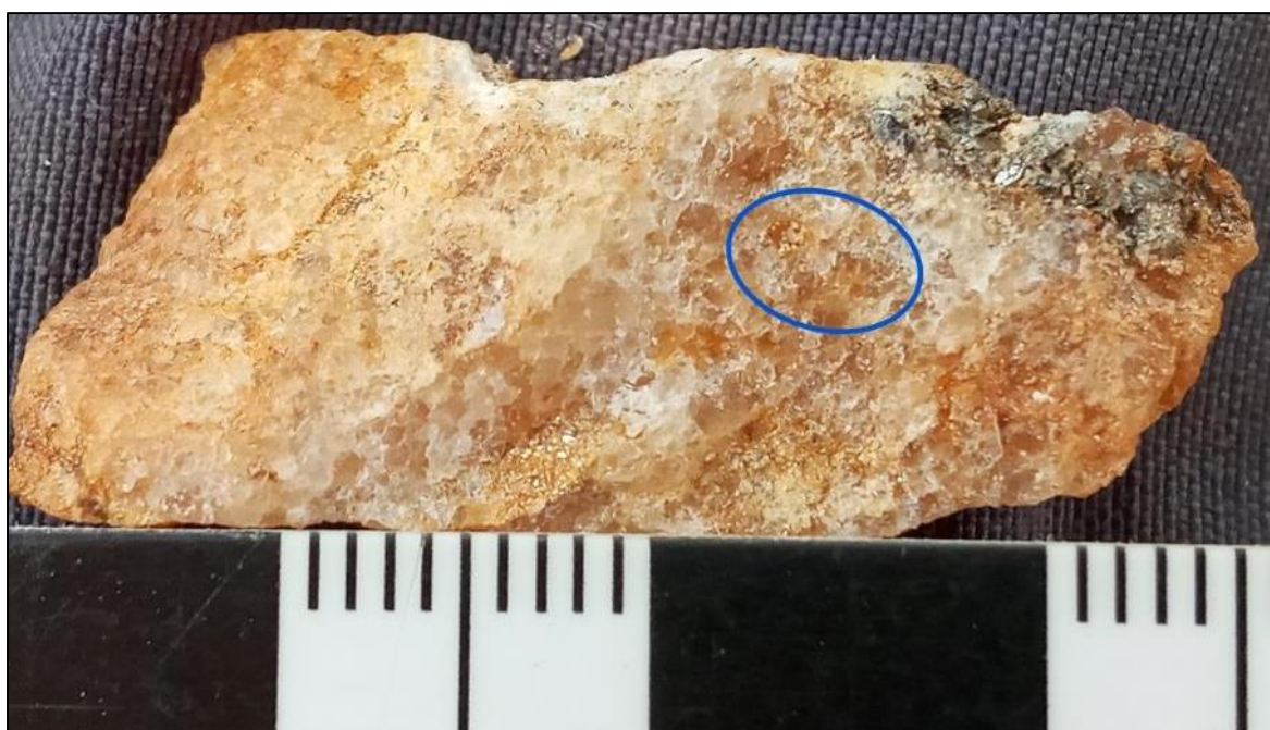
Figure 9: Visible gold in quartz extracted from milky white quartz vein at Chakata
