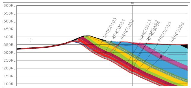
Figure 1. Minex seam model cross-section at the Razorback Iron Project
