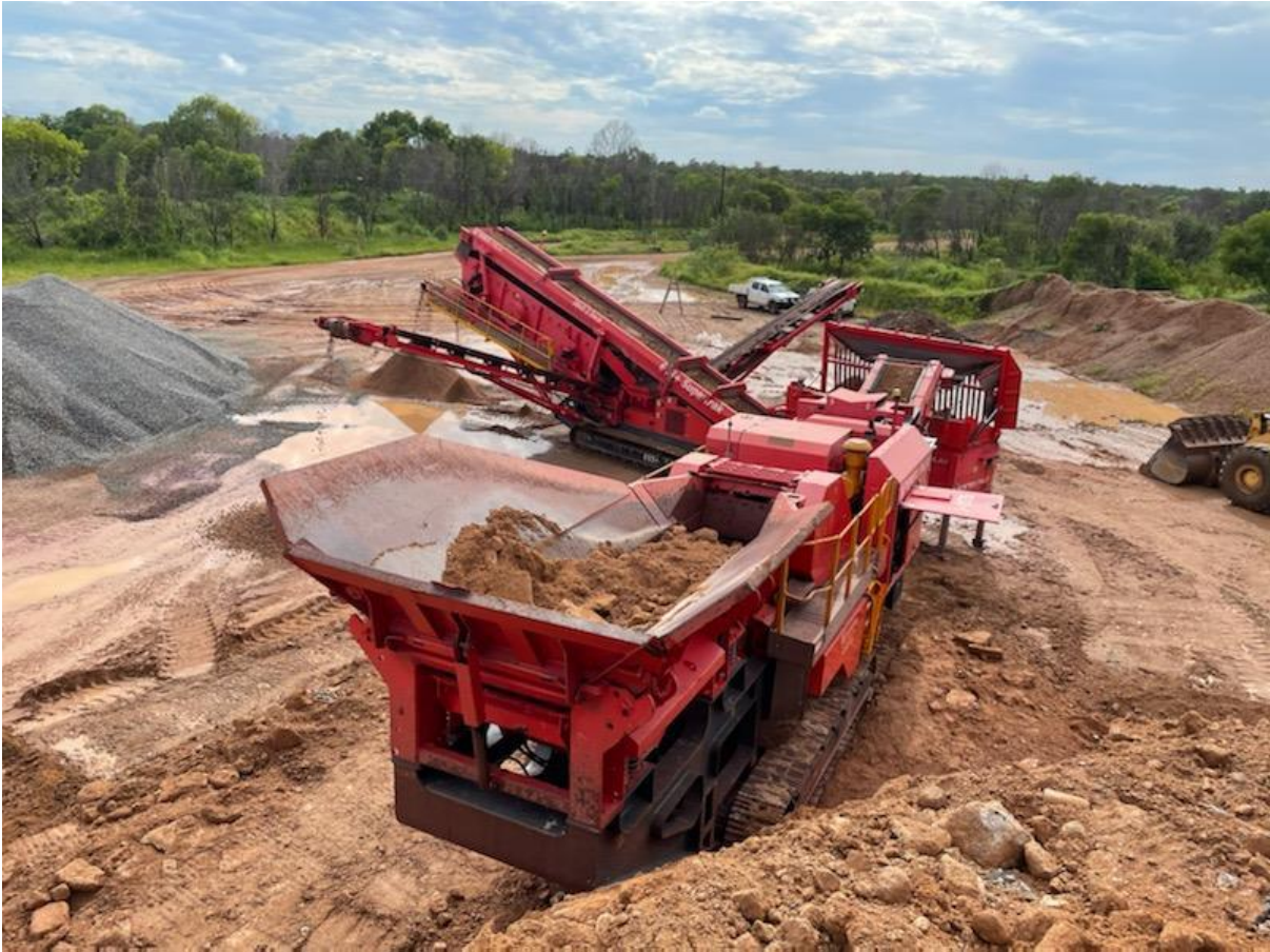
Elmore mobile crushing and screening plant operating near Darwin
