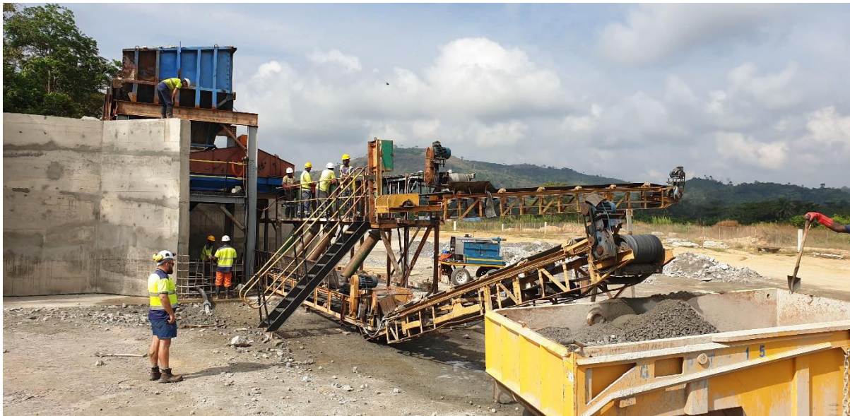
Figure 4: Kimberlite-Waste Sorting Belt
