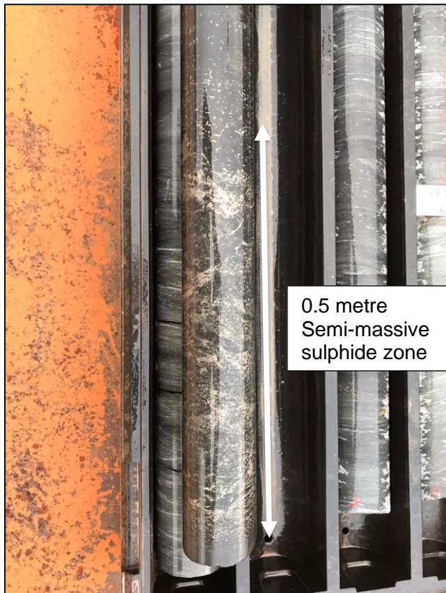
Figure 3 Semi-massive pyrrhotite interval over 0.5 metres
