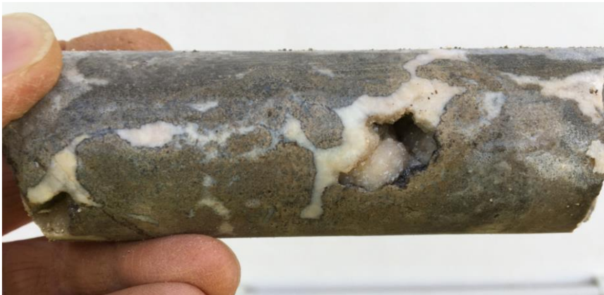
Image 1. Photograph of high-grade sphalerite (zinc) mineralisation from hole NOVDD004 (0 – 1.5m), core diameter 41 mm, located near mine entrance.
