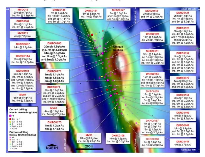
Figure 2 - Plan view highlighting drilling results at Golden Star (source DKM June 2019 Quarterly Report 25/7/19)
