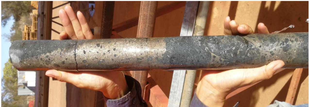
Picture 1. Lower portion of CBDD0042A intersection showing nickel rich sulphides in basal accumulation zone
