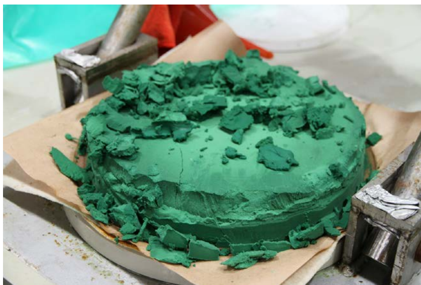
Figure: Mixed Hydroxide Precipitate produced from December pilot plant (currently being refined into battery grade nickel sulfate).
