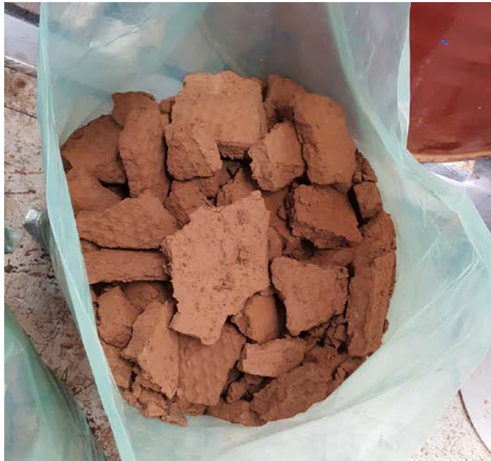
Figure: Leach residue for evaluation as engineered landfill
