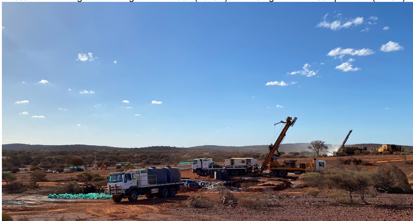
Photo 2: Mt Stirling Diamond rig on MSRD001 (1640N) and RC rig on MSRD002 precollar (1720N)
