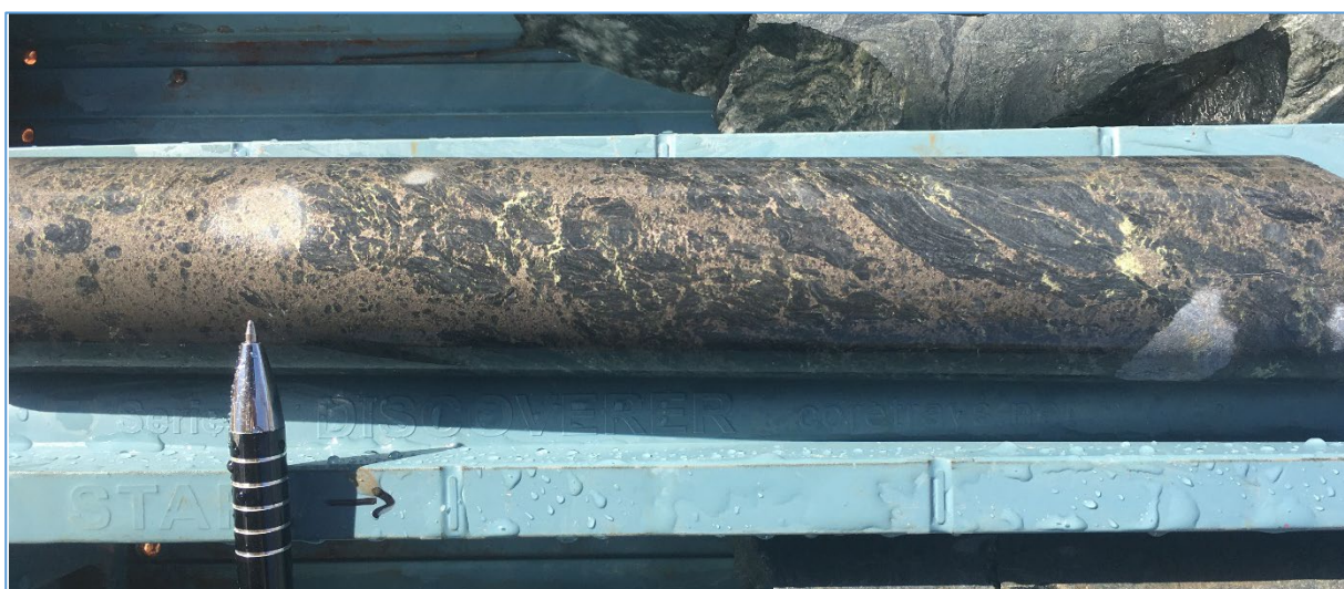
Figure 2: Diamond core from hole 20WD001 at 552.3m showing semi-massive pyrrhotite (bronze colour) and chalcopyrite (yellow) mineralisation.
