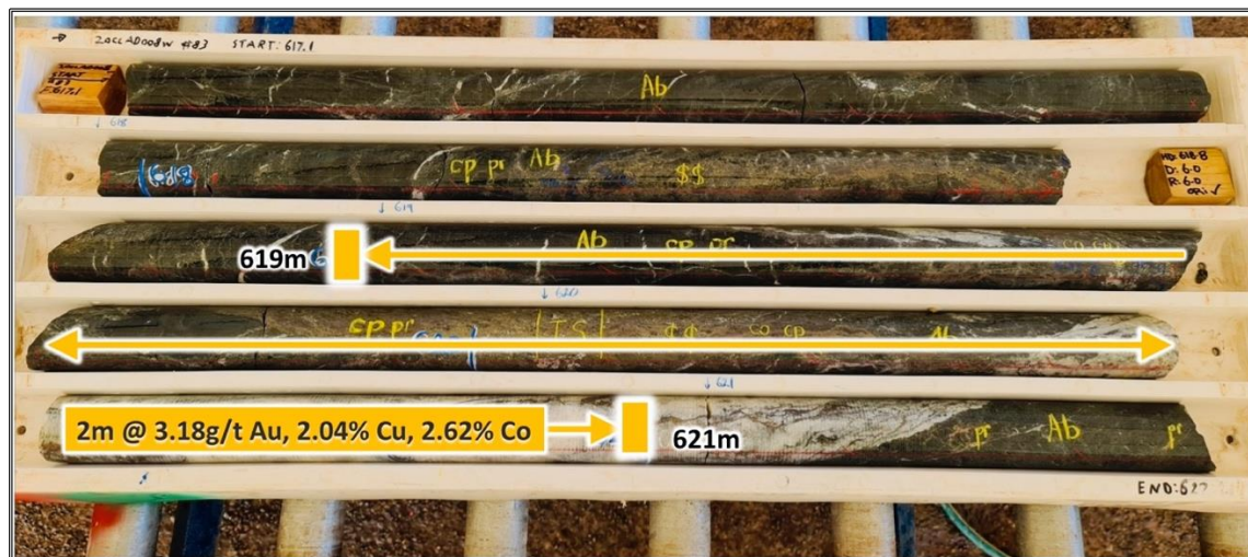
Figure 1: Uncut diamond drill core from hole 20CCAD008W targeting Carlow Deeps. Logged matrix to semi-massive Chalcopyrite, Cobaltite and Pyrrhotite and Pyrite. Final assay results and interval overlain.
