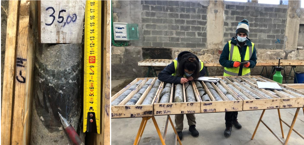
Figures 3 and 4: wolframite vein (4cm) and core from drill hole MC108
