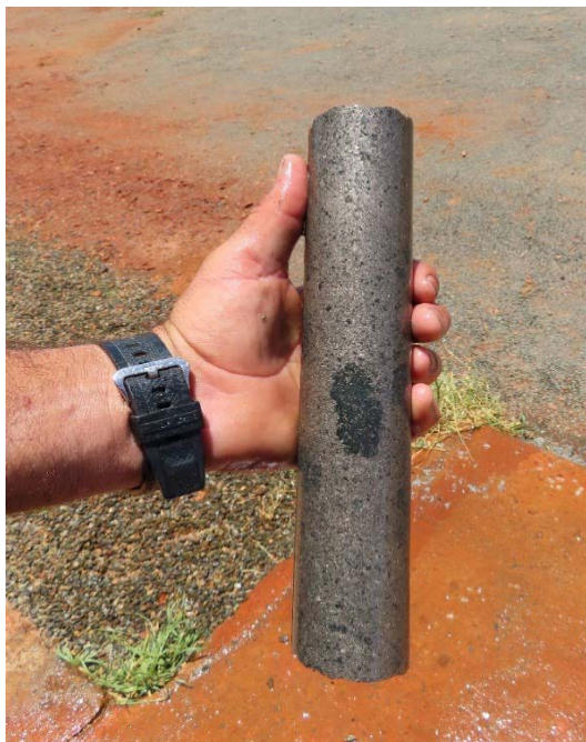
Photo 1: ANDD0012 drill core Massive Ni-Cu sulphides @ 96.0 – 96.2m downhole
