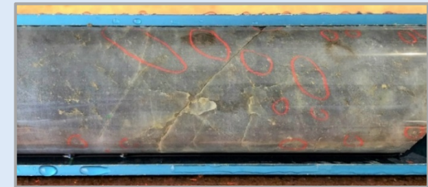
Typical silica-albite-sulphide Tura Lode mineralisation in BBRD1135 at 246.70m (assaying 184.64g/t Au); Multiple clusters of fine visible gold are circled in red; Core diameter is 47.60mm*
