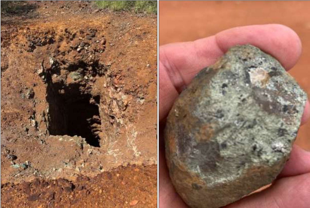
Figure 6: Old shaft at Victory, to the south of Trafalgar (left) and massive sulphides from these workings (right)
