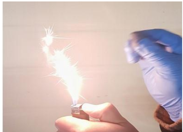
b) ASM’s Ti powder sparks bright orange, indicating high quality due to low oxygen
