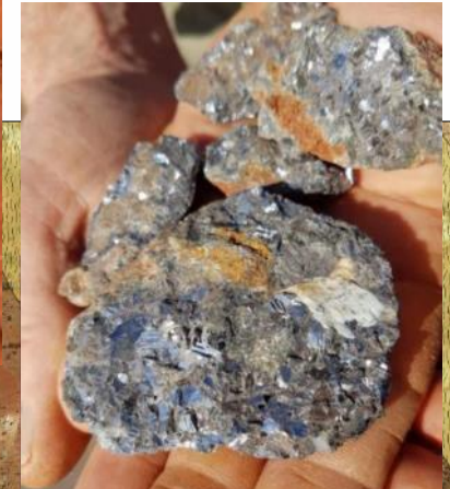
Fresh Galena (Lead Sulphide) approx. 80cm from surface beneath hardpan. 73% Pb, 1,800 g/t Ag
