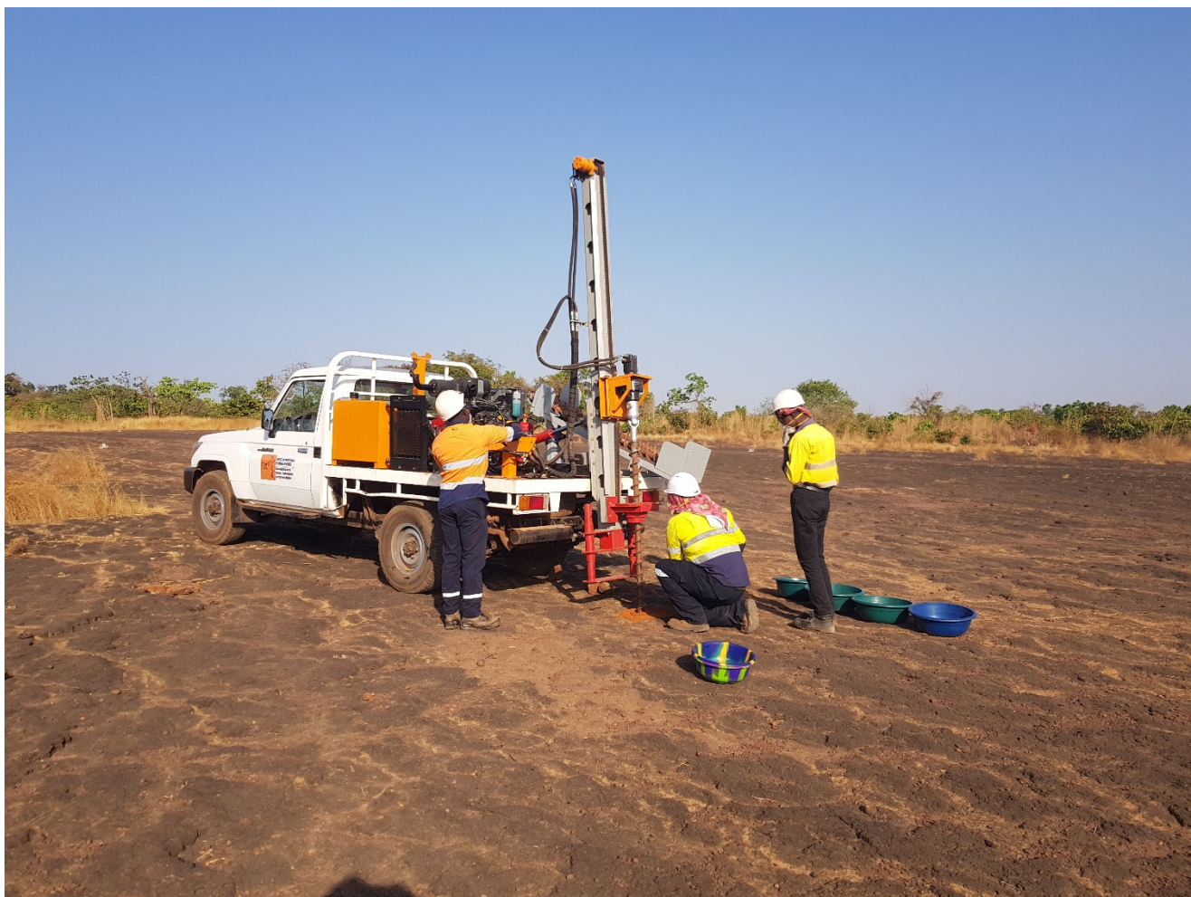
Photo: Auger drilling activities on the Kouroussa Permit
