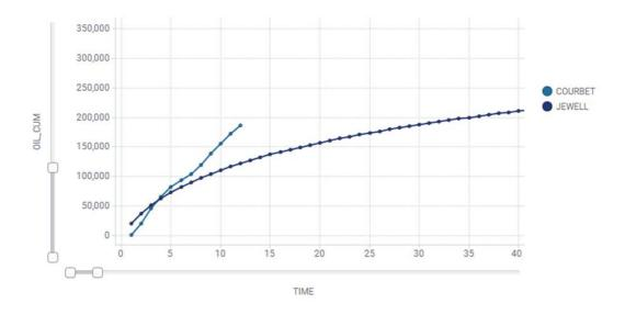
Figure 3: Courbet well cumulative oil production (barrels of oil) versus time (month) compared to the Jewell Well oil production type curve. Brookside has been very conservative in its production estimate for the Jewell Well producing from the Woodford formation.
