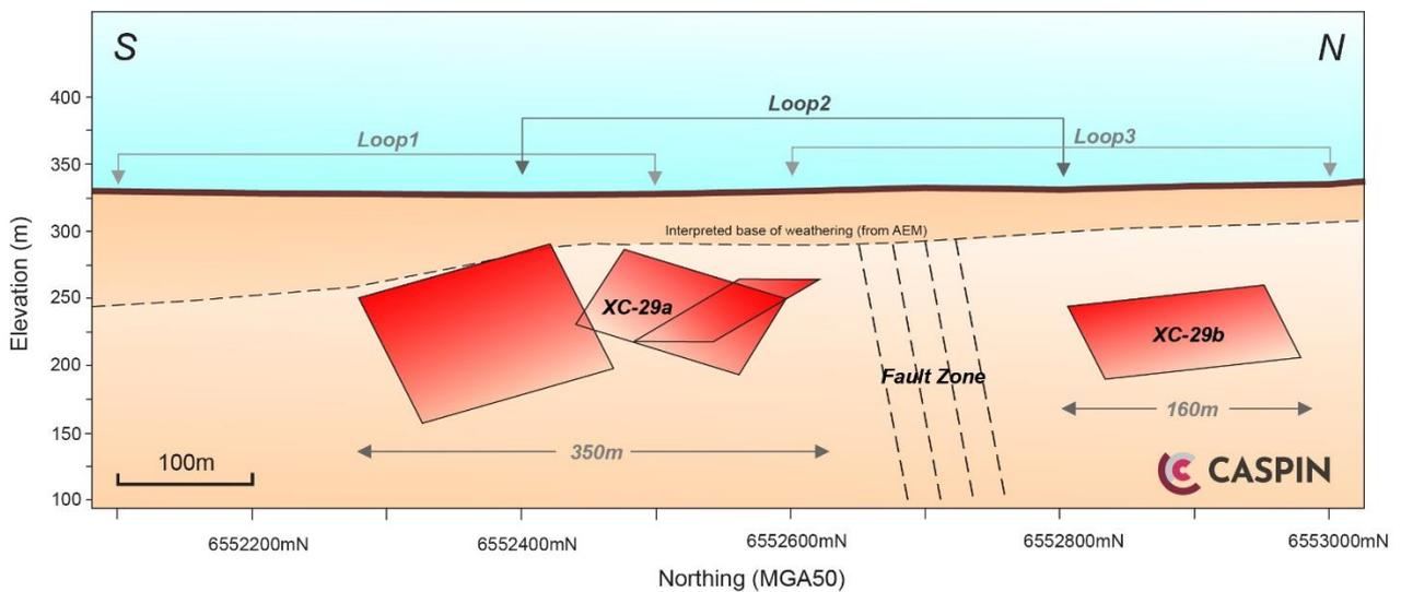
Figure 2. Long section through XC-29a & b showing geometry of FLTEM conductive plates.
