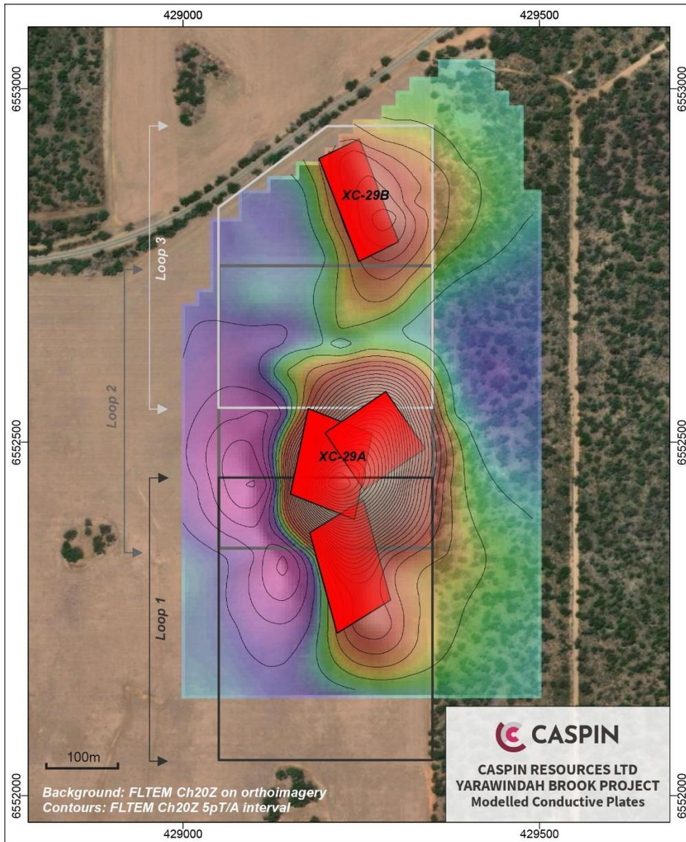
Figure 1. Modelled FLTEM conductors at XC-29a and XC-29b.
