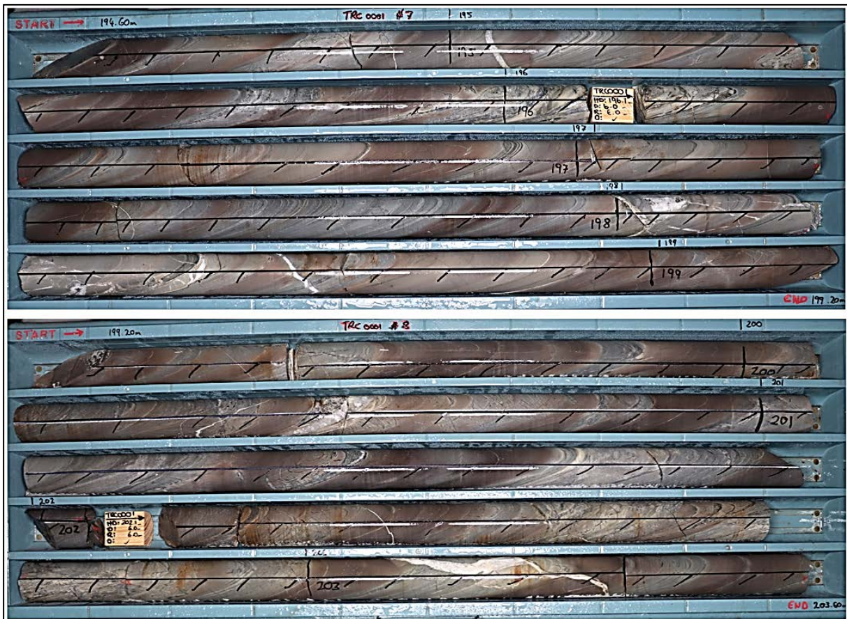
Figure 3: Section of core from TRC0001 from 194.6m to 203.6m showing intensity and vein styles with alteration in volcanoclastic sediments.
