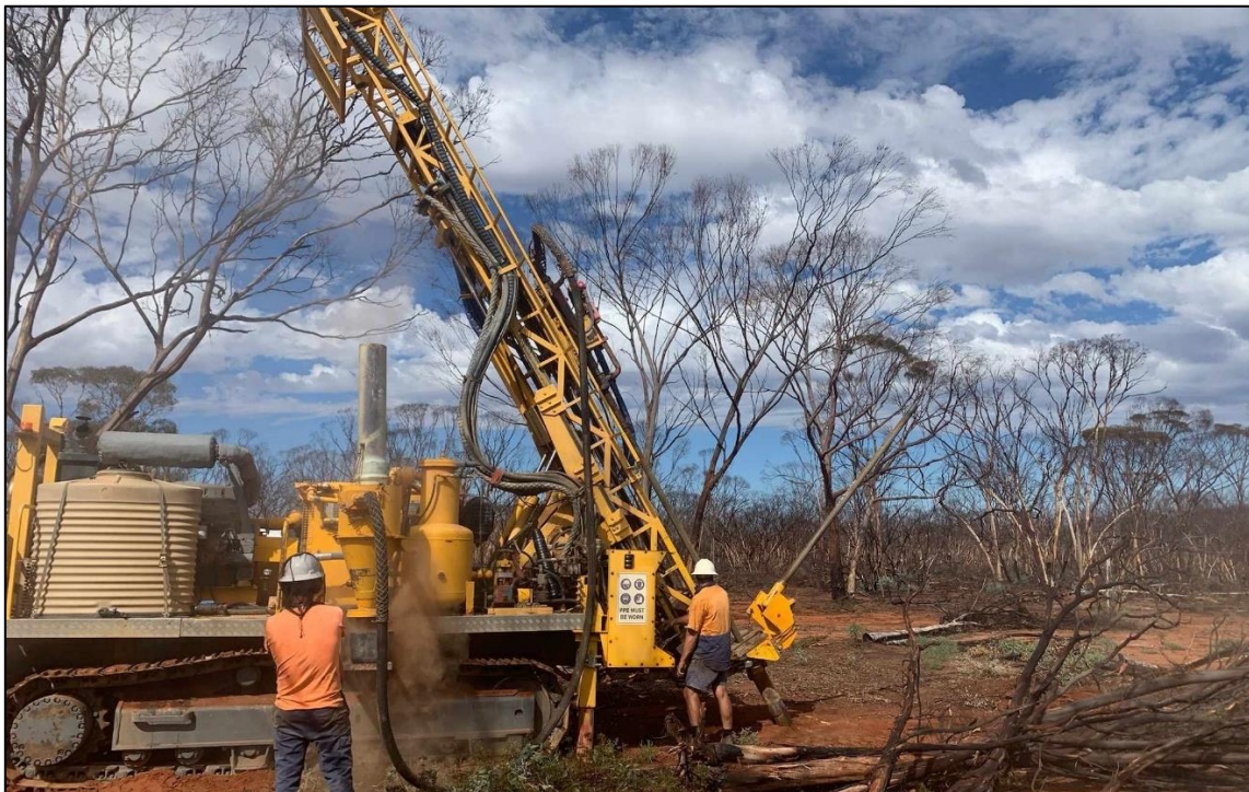
Figure 1 - Nepean Nickel-Gold Project, maiden air-core drilling program underway.
