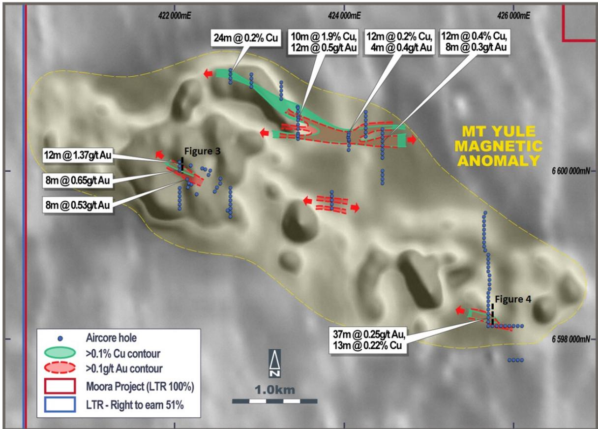
Figure 2: Mt Yule Prospect – Drill hole plan on magnetic image showing better aircore results.
