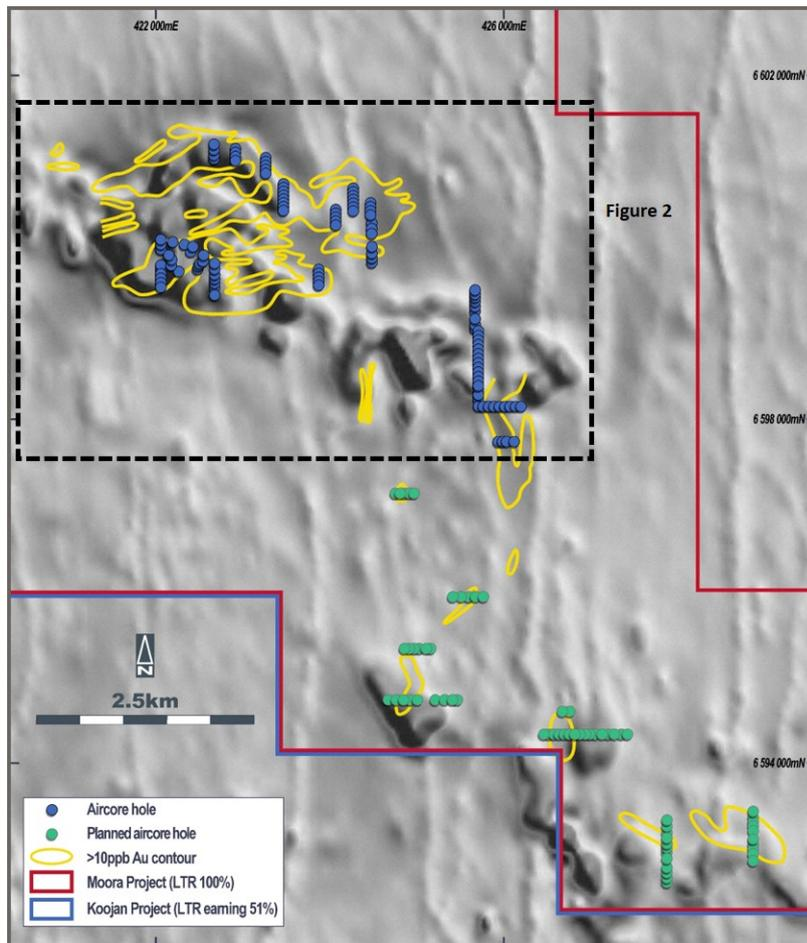
Figure 5: Drill hole plan on grey scale magnetic image.
