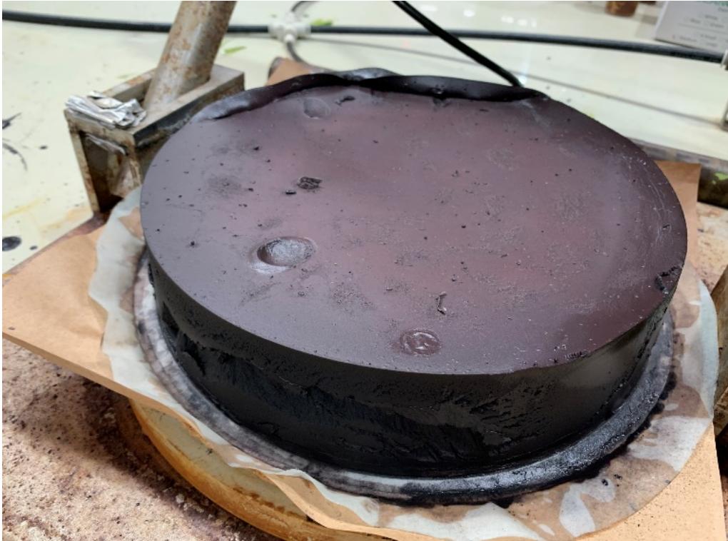
Figure: Precipitated iron from pilot plant
