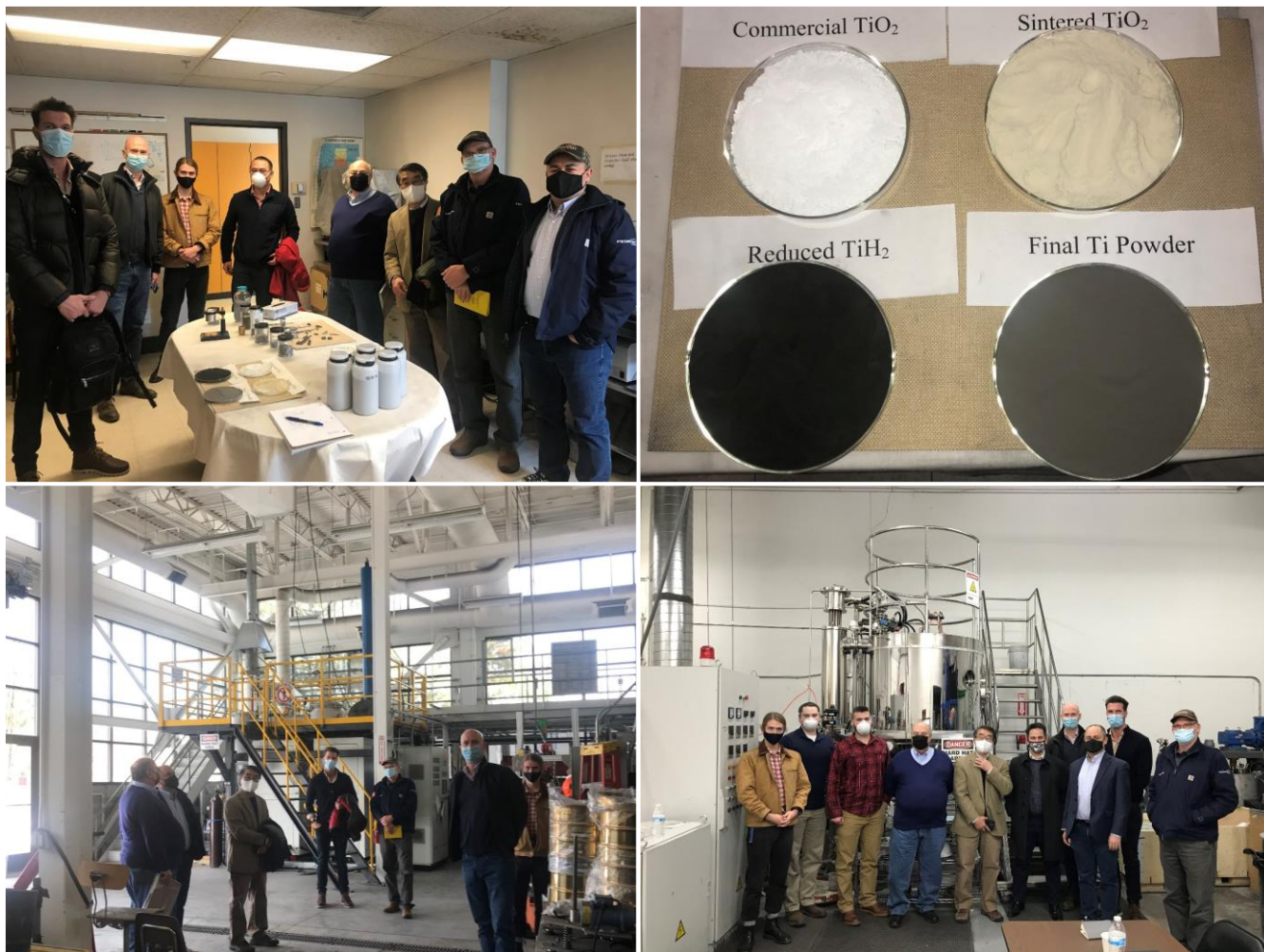
Figure 9: From top left, Blacksand and TAO team in product analytical lab at the University of Utah, \text{TiO}_2 powder to Ti powder, Pilot scale furnace in University of Utah, team at Blacksand Laboratory
