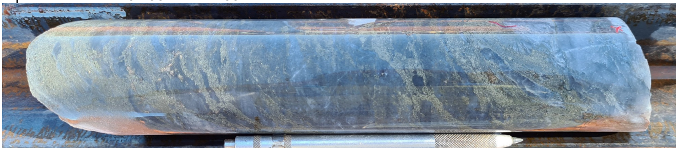
Photo 1: MSRD005 Detailed lode mineralisation with up to 15% pyrite and pyrrhotite sulphides representative of 261.36m – 271.00m
