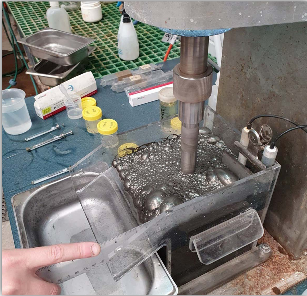
Flotation Test Work of RKDD034 Massive Sulphide
